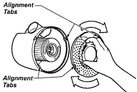
Rotate filter screen clockwise to lock in place.
